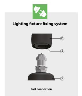
An axle box is welded to the pole arm (A) to allow the fast connection of the Ghisamestieri lighting fixture (X). A die-cast aluminium decoration (D) hide the fixing system.
