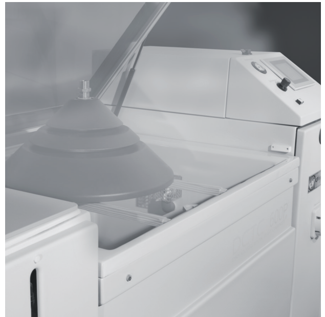
Test nebbia salina | FLORIDA TEST
