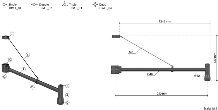
Pole arm predisposed for the installation of suspended lighting fixtures. Available in single, double, triple or quad versions on 7-8-9-10 m. poles. The pole arm is equipped for the pole fixing and for the suspended lighting fixtures fixing.
