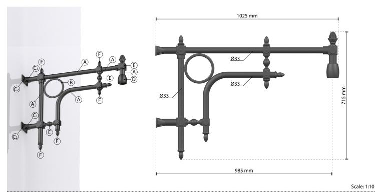
Wall bracket predisposed for the installation of suspended lighting fixtures. The wall bracket is equipped for the suspended lighting fixtures fixing.
