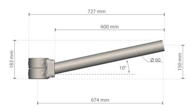
The drawings show the pole arm with Ø 89 pole collars, suitable for Steel Black poles fixing. The pole arm is equipped with Ø 79 pole collars for Steel Red or Steel Green poles fixing. (Ø 79 pole collars are shown in the pictures at the bottom.)
