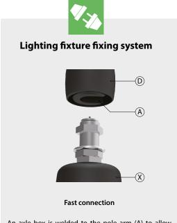
An axle box is welded to the pole arm (A) to allow the fast connection of the Ghisamestieri lighting fixture (X). A die-cast aluminium decoration (D) hide the fixing system.
