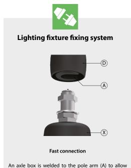
the fast connection of the Ghisamestieri lighting fixture (X). A die-cast aluminium decoration (D) hide the fixing system.
