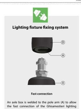
fixture (X). A die-cast aluminium decoration (D) hide the fixing system.
