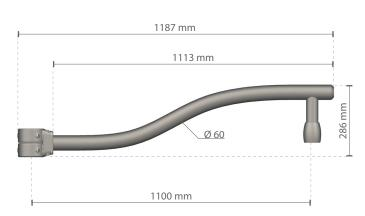
The drawings show the pole arm with Ø 89 pole collars, suitable for Steel Black poles fixing. The pole arm is equipped with Ø 79 pole collars for Steel Red or Steel Green poles fixing. (Ø 79 pole collars are shown in the pictures at the bottom.)
