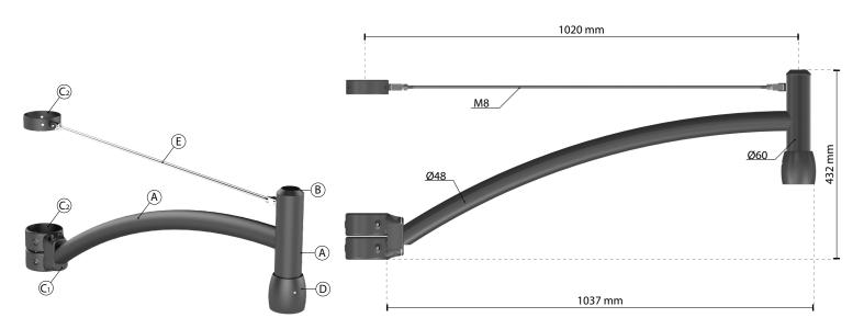
Pole arm predisposed for the installation of suspended lighting fixtures. Available in single or double versions on 5-6 m. poles. The pole arm is equipped for the pole fixing and for the suspended lighting fixtures fixing.
