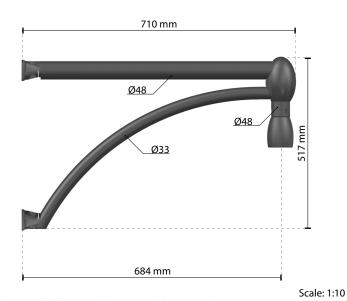
Wall bracket predisposed for the installation of suspended lighting fixtures. The wall bracket is equipped for the suspended lighting fixtures fixing.
