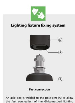
An axle box is welded to the pole arm (A) to allow the fast connection of the Ghisamestieri lighting fixture (X). A die-cast aluminium decoration (D) hide the fixing system.
