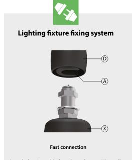
An axle box is welded to the pole arm (A) to allow the fast connection of the Ghisamestieri lighting fixture (X). A die-cast aluminium decoration (D) hide
