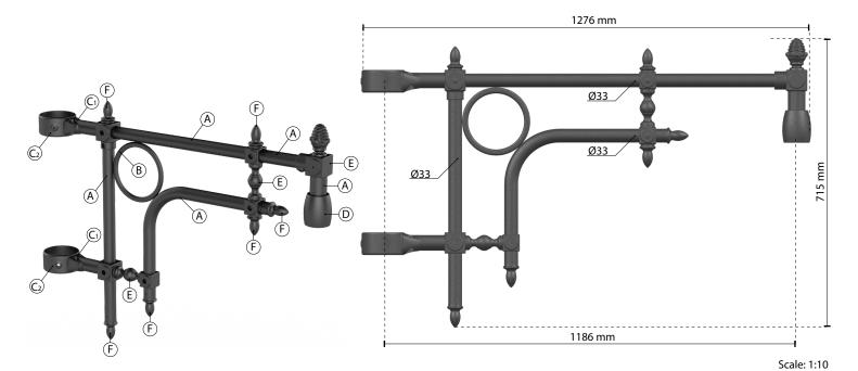
Pole arm predisposed for the installation of suspended lighting fixtures. Available in single or double versions on 5-6 m. poles. The pole arm is equipped for the pole fixing and for the suspended lighting fixtures fixing.
