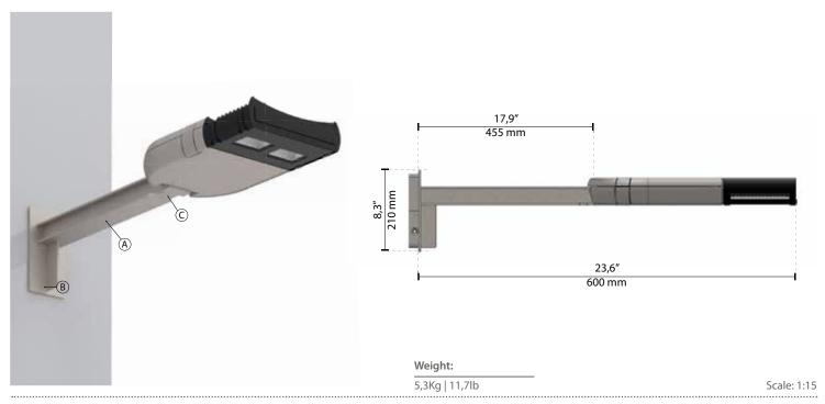
Wall bracket predisposed and equipped for the installation of Izar small lighting fixture with lateral fixing.
