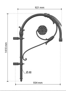
Pole arm predisposed for the installation of suspended lighting fixtures. Available in single, double, triple or quad versions on 7-8-9-10 m. poles. The pole arm is equipped for the pole fixing and for the suspended lighting fixtures fixing.
