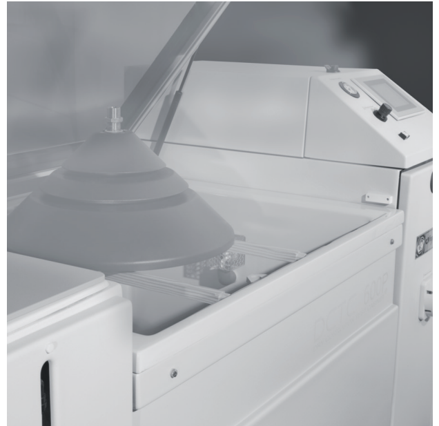
Salt spay test | FLORIDA TEST
