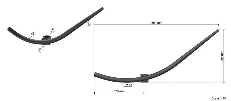
Pole arm predisposed for lighting fixtures lateral fixing. Available in single or double versions on 7-8-9-10 m. poles. The pole arm is equipped for the pole fixing.
