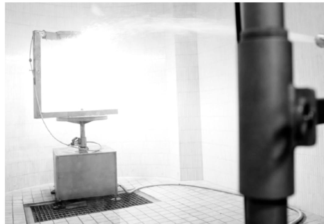
**LABORATORIOS INTERNOS | CÁMARA PARA PRUEBA IP**
